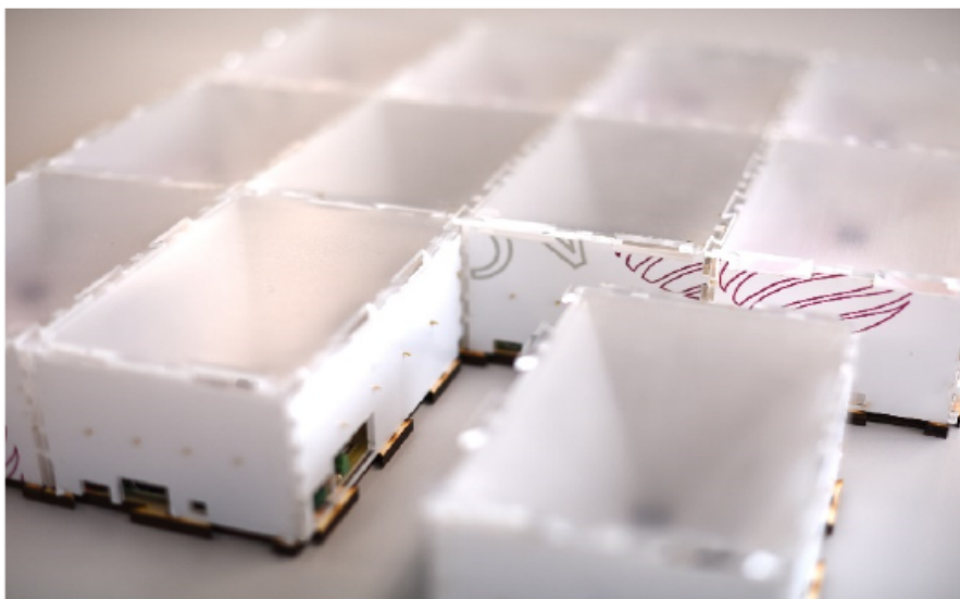
Figure 1. The modular design of an IRIS surface showing the interlocking, tessellating units.
