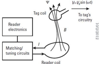
$$\Psi = \int B \bullet dS \qquad V_{T_{dg}} = 2\pi f NQB(S\cos\alpha)$$
