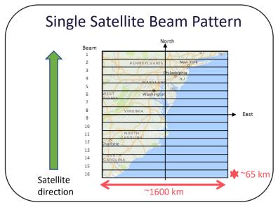
Each satellite has 16 user beams, arranged in a "venetian blind" pattern. The "footprint" of each satellite overlaps slightly with adjacent satellite footprints to create gapless coverage
