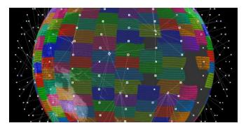
FWD User Beams are assigned downlink frequencies using 8-color reuse Each frequency is used twice among 16 beams
