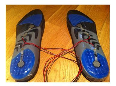
Figure 5.1: Sensors mounted under shoe soles
