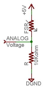
Figure 4.3: Voltage divider circuit
