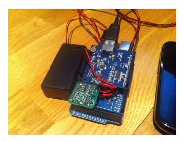
Figure 5.2: Arduino MCU prototyping board, USB host shield, sensor circuit perfboard
