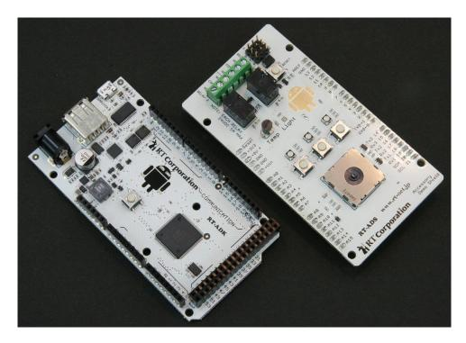
Figure 2.10: Android ADK Demo Shield
