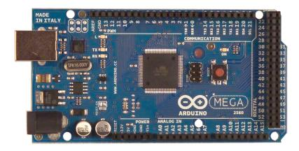
Figure 3.4: Selected MCU prototyping board, Arduino Mega 2560
