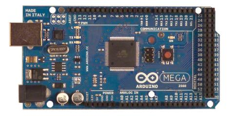
Figure 2.4: Arduino Mega 2560
