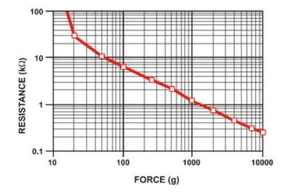
Figure 3.8: Resistance at different force measurements
