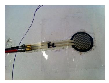
Figure 4.1: FSR with soldered pins
