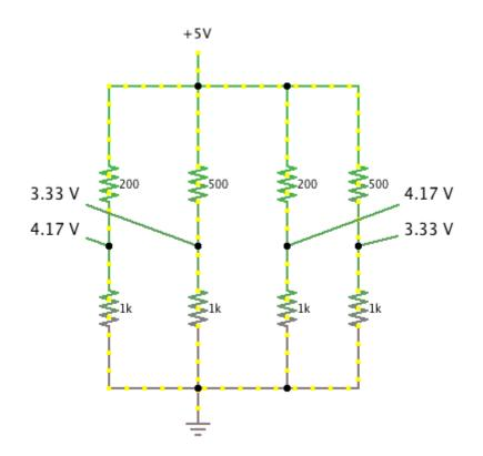
Figure 4.4: Four voltage divider circuits
