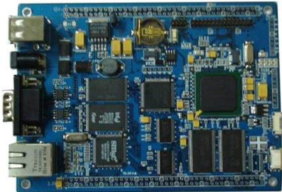
PCB Standard with PXA270 110x130mm WCP ~ 350Euro
