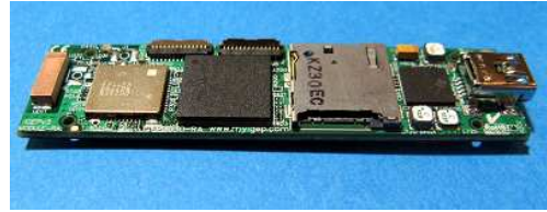
PCB OMAP (18x68mm) Computational Power 5X WCP (1K pcs) = ~ 100 Euro
