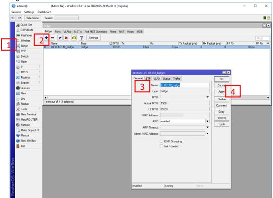
6. Then, add "wlan1" and "ether1" to the bridge interface that you have created in previous step.
