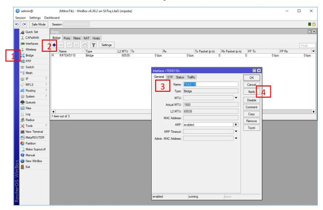
4. Then, add "wlan1" and "ether1" interfaces to the bridge interface so that device that connects to Ethernet interface can connect to RB921GS network.
