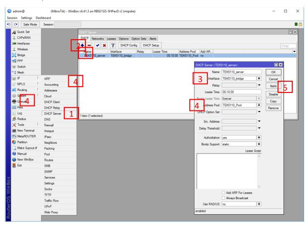
10. Finally, we need to define DHCP server's options (network, gateway and DNS servers) and finish configuration of RB921GS as a P2P wireless access point.
