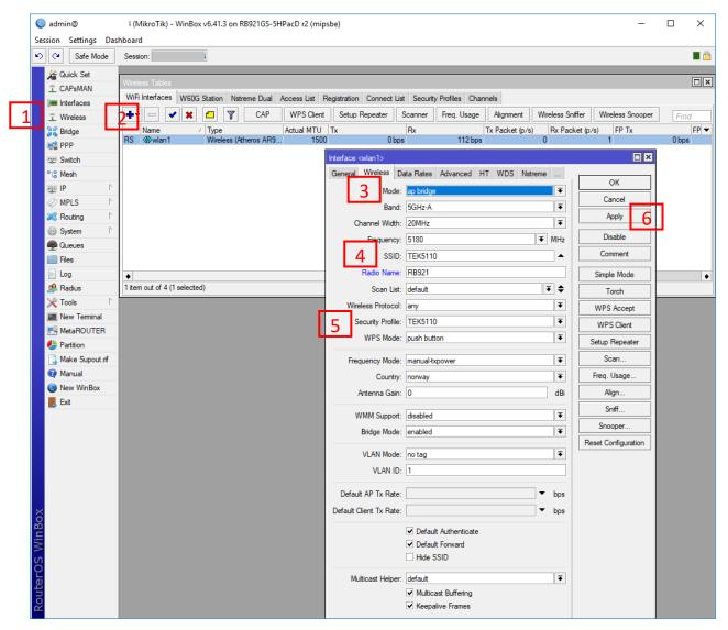
5. Now, create a bridge interface "TEK5110" in order to connect wireless and Ethernet interfaces together.
