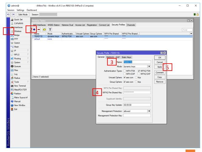
4. Then, enable "wlan1" interface and configure wireless interface to be access point bridge. In the Wireless tab, select an SSID e.g. "TEK5110" and select security profile "TEK5110" that you have created in previous step.
