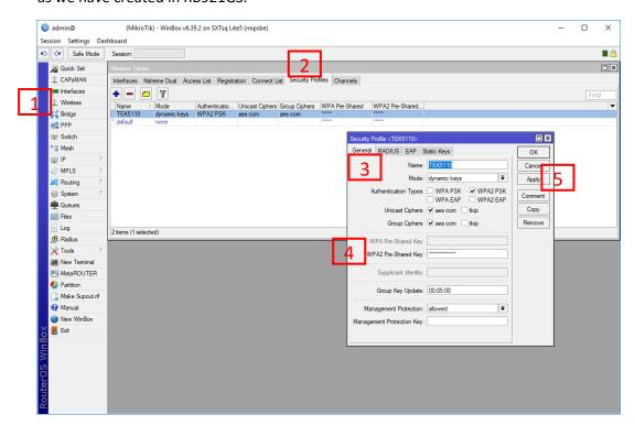
1. Then, we can configure "wlan1" interface to be as a station bridge interface so that it can connect its clients in the ethernet port to P2P wireless network. In addition, you should select RB921GS SSID "TEK5110" and security profile "TEK5110" that you have created in previous step.
