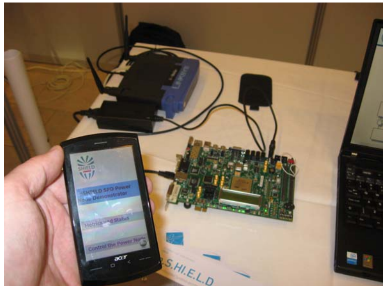
Figure 4 – Running FPGA Power Node Prototype
