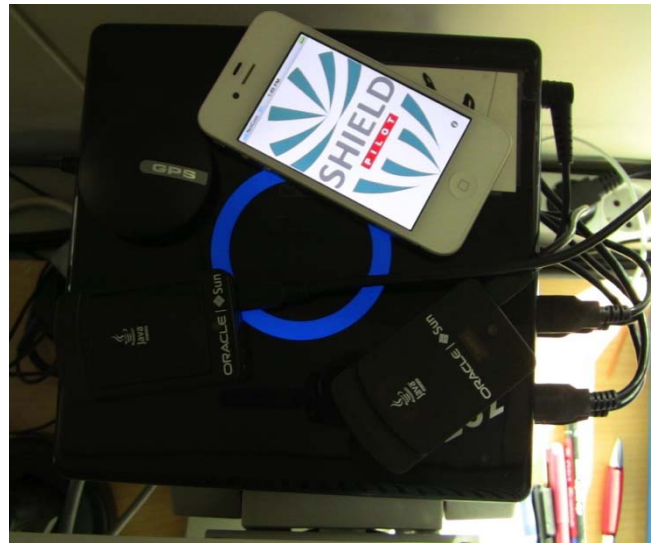
Figure 26 - The embedded platform with the Sun SPOT host, the Sun SPOT sensor and the GPS
