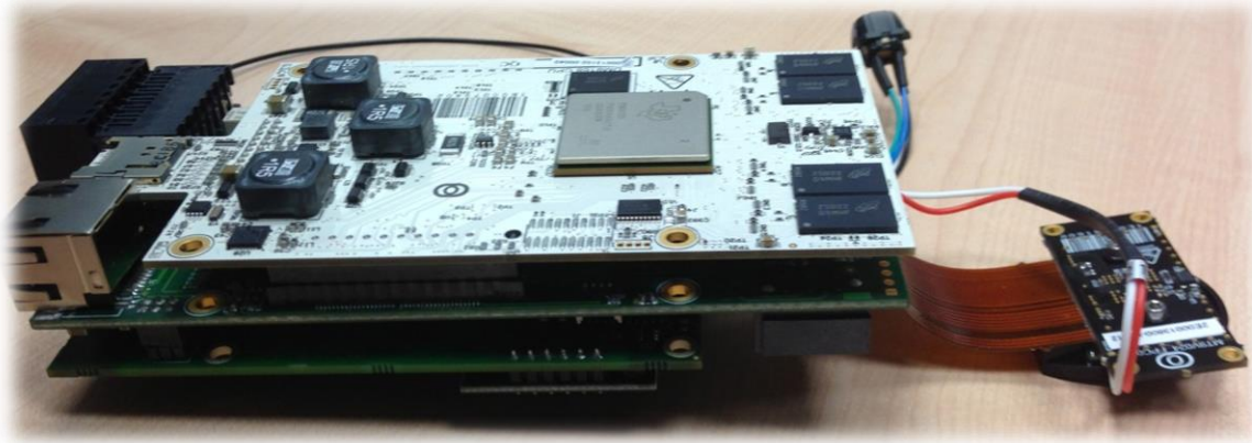
Figure 3-3: The custom embedded board based on TI SoC
