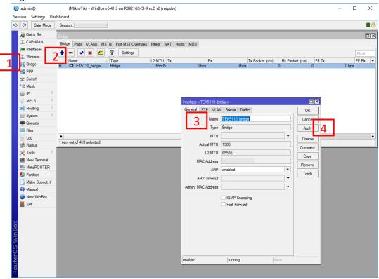
6. Then, add "wlan1", "wlan2" and "ether1" to the bridge interface that you have created in previous step.
