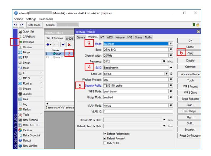
5. Now, create a bridge interface "TEK5110" in order to connect wireless and Ethernet interfaces together.
