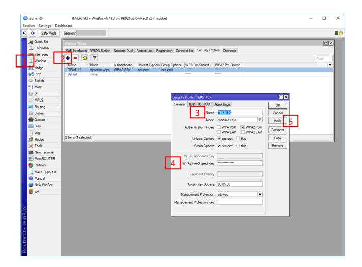
4. Then, enable "wlan1" and "wlan2" interface and configure wireless interface to be access point bridge. In the Wireless tab, select an SSID e.g. "BasicInternet" and select security profile "TEK5110" that you have created in previous step.
