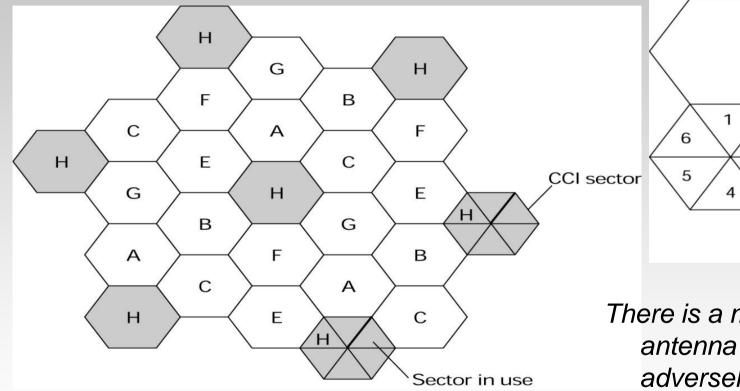
There is a major drawback on sectorized antenna approach to improving S/I ratio- it adversely affect the overall capacity of the system. This can be explained using the concept of trunking.
