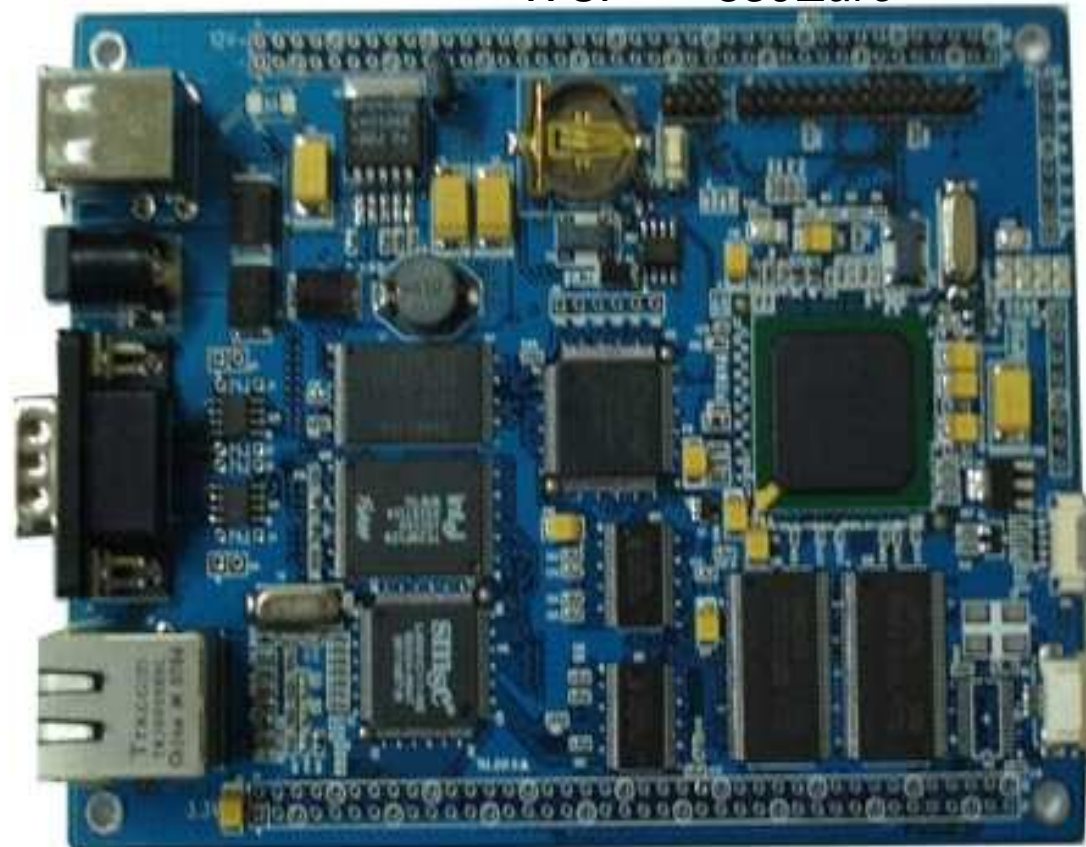
PCB OMBRA-nSHIELD (18x68 mm) OMAP uP, Xilinx FPGA WCP (1K pieces) = ~150 Euro Computational Power 5X
