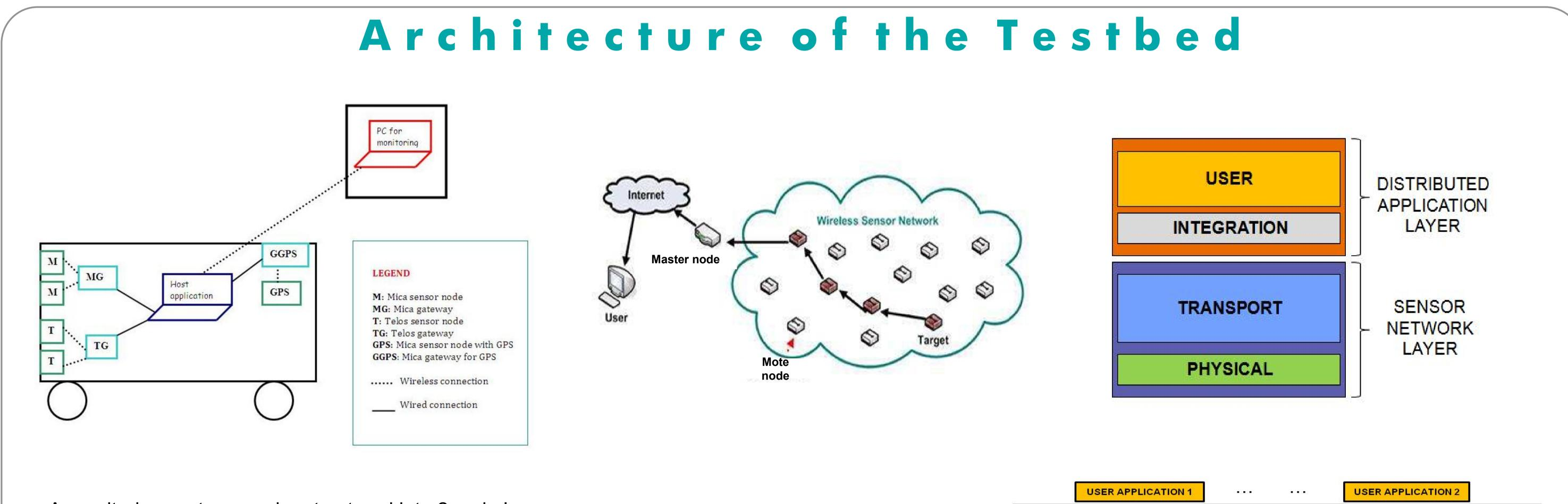
A monitoring system can be structured into 2 main layers:
