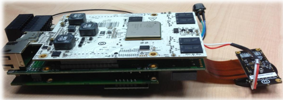
Figure 3-8: The custom embedded board based on TI SoC.
