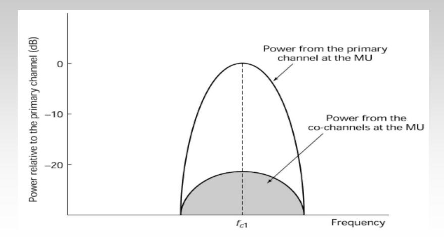
Signal to noise ratio can be defined:  $\frac{S}{N} = \frac{\text{signal power}(S)}{\text{noise power } (N_s) + \text{ interfering signal power } (I)}$
