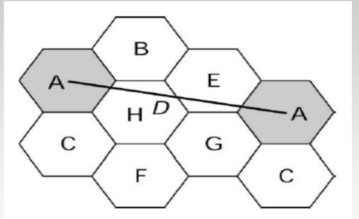
In hexagonal geometry, there are six neighbors of each cell and the line joining the centers of any cell and each of its neighbors are separated by 60 degrees. This restricts the number of usable cluster sizes and their layouts. In order to *tessellate*-to connect cells without gap-the number of cells per cluster, N, can only have values, which satisfy the following equation:
