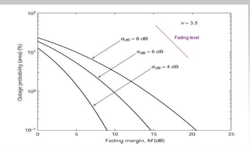
Outage goes up as fading level increases (at fixed fade margin)
