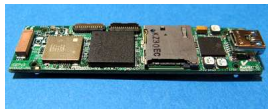
PCB OMAP (18x68 mm) WCP (1K pcs) \approx 100 Euro Computational Power 5X
