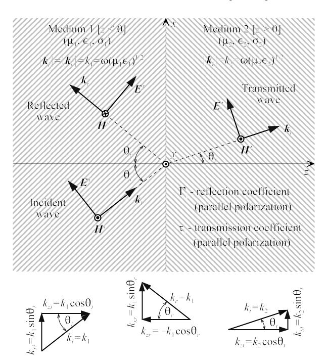
Using the basic concepts of the reflection and transmission coefficients, the phasor electric and magnetic fields associated with the incident, reflected and transmitted waves may be written as
