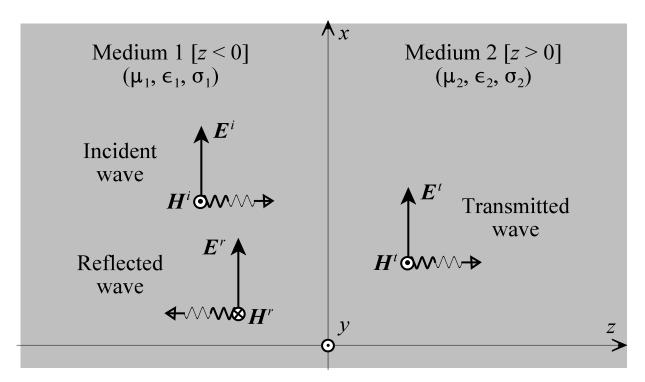
Enforcement of the boundary conditions (continuous tangential electric field and continuous tangential magnetic field) yields
