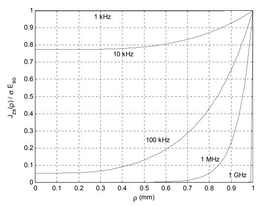
As frequency increases, the current becomes concentrated along the outer surface of the wire.
