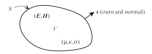
The quantity under the integrand on the left hand side of Poynting's theorem is defined as the Poynting vector.
