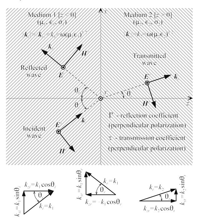
The electric and magnetic fields of the incident, reflected and transmitted waves in the case of perpendicular polarization are
