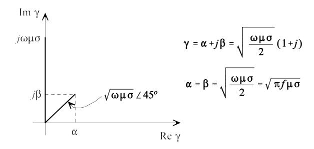
Note that attenuation in a good conductor increases with frequency. The rate of attenuation in a good conductor can be characterized by a distance defined as the *skin depth*.
