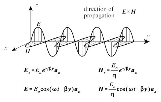
Note that the electric field and magnetic field in a lossless medium are in phase.
