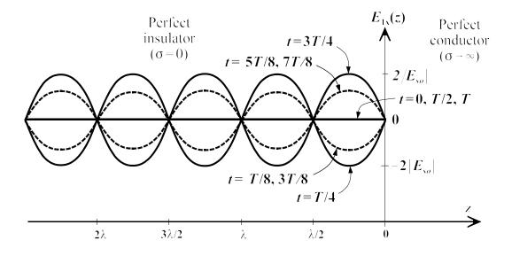
The locations of the minimums and maximums of the standing wave electric field pattern are found by
