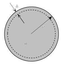
The equivalent model is a ring of uniform current density along the outer surface of the conductor (depth equal to one skin depth).
