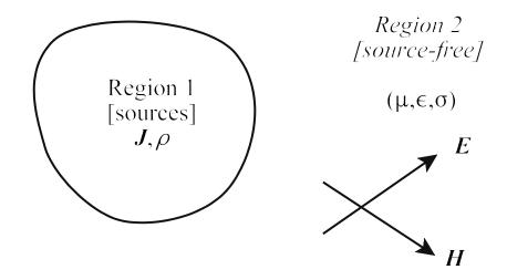
We start with the source-free, instantaneous Maxwell's equations written in terms of E and H only. Note that conduction current in the source-free region is accounted for in the  $\sigma E$  term.
