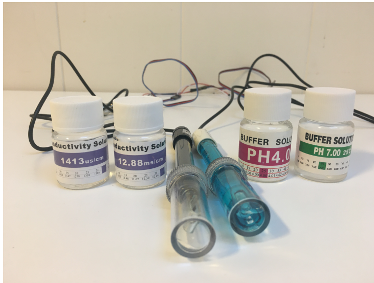
Figure 23: EC, pH probes and standard buffer calibration solutions
