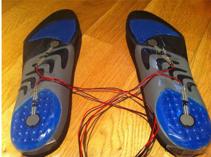
Figure 5.1: Sensors mounted under shoe soles
