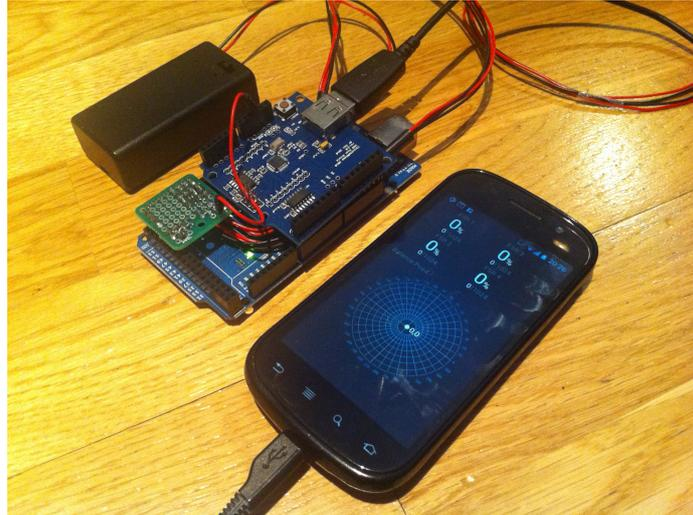
Figure 5.3: Android mobile phone connected to Arduino
