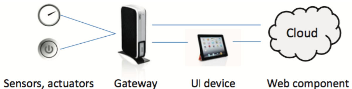
Figure 2.2: Elements of an IoT Application [Oleksiy & Passi, 2014]
