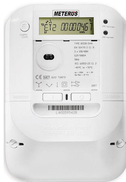
Figure 4.2: Example of a smart meter based on Open Smart Grid Protocol (OSGP) [ETSI, 2012] in use in Europe that has the ability to reduce load, disconnect-reconnect remotely, and interface to gas and water meters. Picture is taken from [Smart Meter, 2016].
