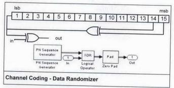
The generator defined for the randomizer is given by Equation (1)  $1 + x^{14} + x^{15}$  (1)
