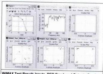
WiMAX Test Result: Inputs, BER Graph and Outputs Graphs
