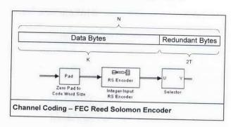
WiMAX uses a fixed RS Encoding technique based on  $GF(2^8)$  which is denoted as RS(N = 255, K = 239, T = 8)
