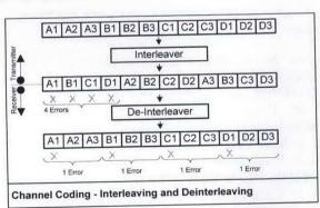
The block interleaver interleaves all encoded data bits with a block size corresponding to the number of coded bits per OFDM symbol. The number of coded bits depends on the modulation technique used in the Physical layer. WiMAX 802.16e supports 4 modulation techniques and is adaptive in the selection of a particular technique based on the channel conditions and data rate.
