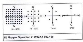
The constellation-mapped data is subsequently modulated onto all allocated data carriers in order of increasing frequency offset index.
