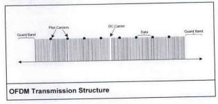
Guard band, pilot carriers and DC carrier are inserted in the structure before using the IFFT to convert the frequency domain signals into time domain. These time domain signals are then transmitted through the channel.
