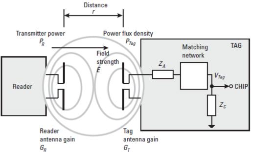
$E^{2}/120\pi = P_{R}G_{R}/4\pi r^{2}$   $P_{Tag} = (E^{2}/120\pi)(\lambda^{2}/4\pi)G_{T} = V_{tag}^{2}/R_{c}$   $P_{Tag} = (P_{R}G_{R}/4\pi r^{2})(\lambda^{2}G_{T}/4\pi) = P_{R}G_{R}G_{T}\lambda^{2}/(4\pi)^{2}r^{2}$   $V_{Tag} = (\lambda/4\pi r)\sqrt{P_{R}G_{R}G_{T}R_{c}}$ Device trapeptitted is regulated by ECC (in EIDD) and CE
