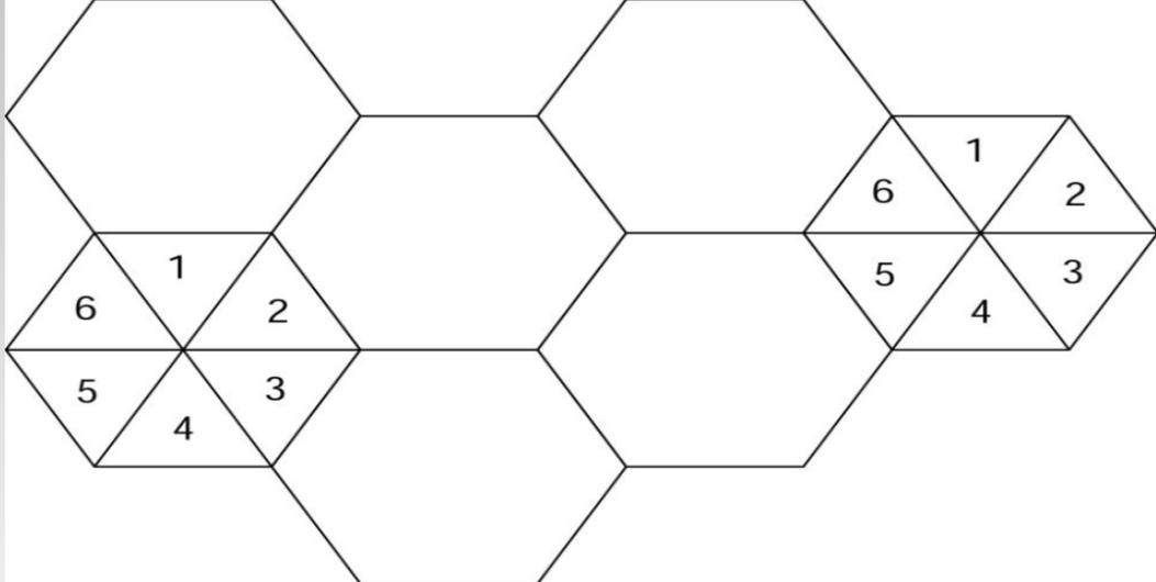
*There is a major drawback on sectorized antenna approach to improving S/I ratio- it adversely affect the overall capacity of the system. This can be explained using the concept of trunking.*
