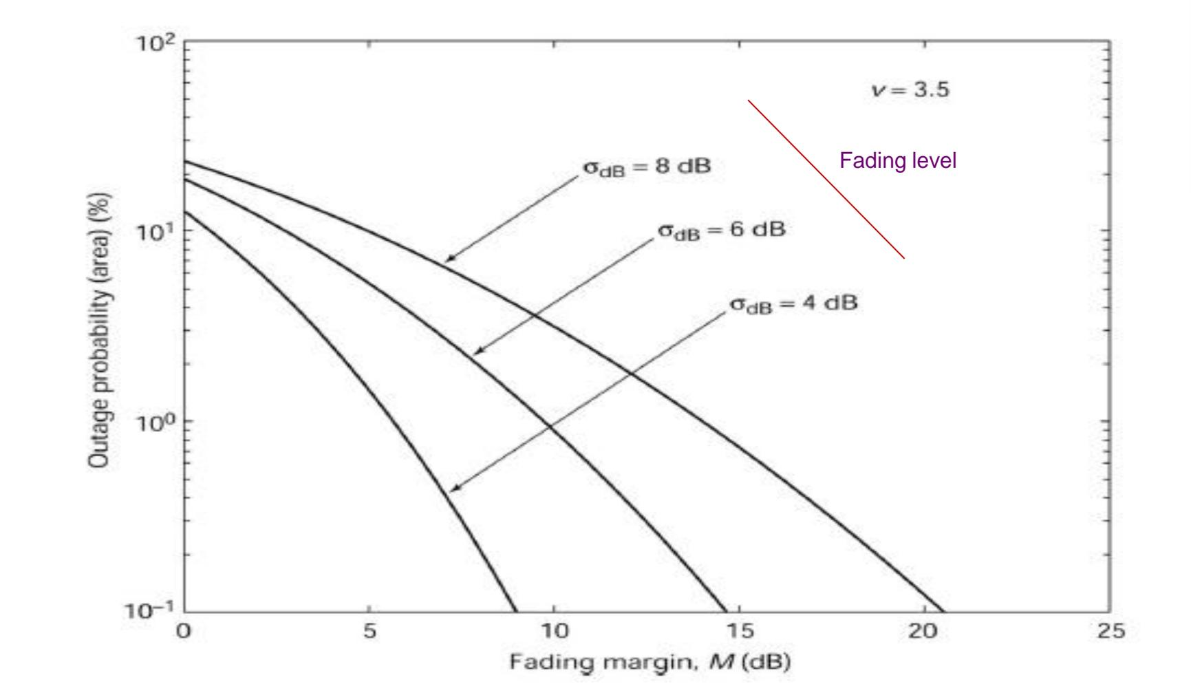
Outage goes up as fading level increases (at fixed fade margin)
