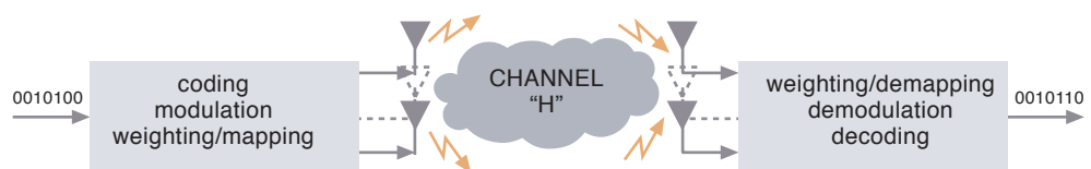
Figure 1 Diagram for a MIMO wireless transmission system. The transmitter and receiver are equipped with multiple antenna elements. Coding, modulation and mapping of the signals onto the antennas may be realized jointly or separately
